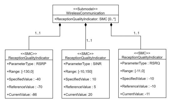
Figure 7: Example of use of the Submodel ReceptionQuality for 5G.
