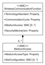
Figure 4: UML-Diagram of the Submodel collection "WirelessCommunicationFunction".
