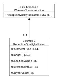
Figure 9: Example of use of the Submodel ReceptionQuality for WirelessHART.
