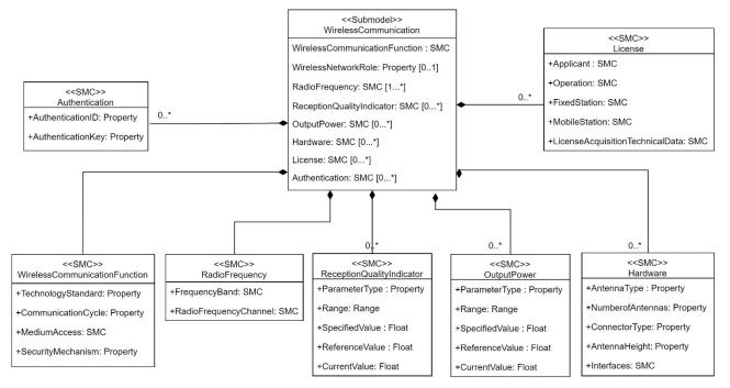
Figure 3: UML-diagram of Submodel WirelessCommunication.
