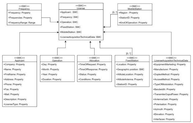
Figure 6: UML-Diagram of the Submodel collection "License".
