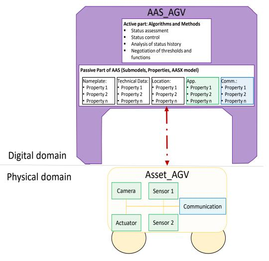
Figure 1: Asset and AAS of an AGV.
