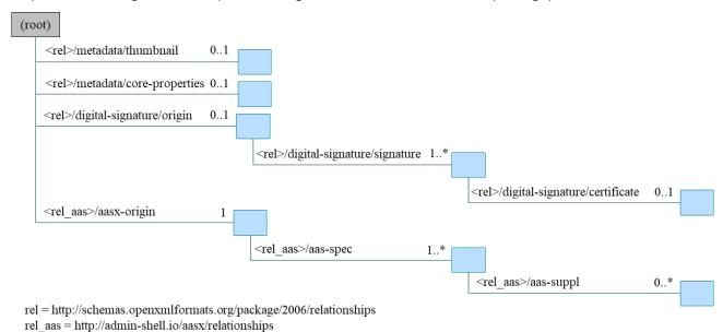
Figure 7 Relationship Types for AASX Packages (Logical Model)
