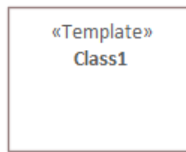
Figure 44 Graphical Representation of a Template Class
