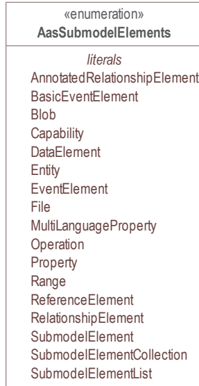
Figure 51 Metamodel of AasSubmodelElements Enumeration
