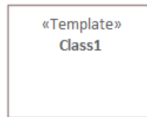
Figure 87 Graphical representation of a Template Class
