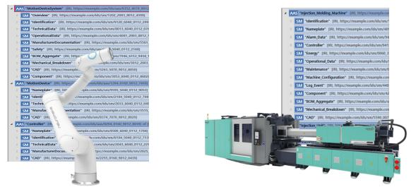
Fig. 1 AAS of the collaborative robot arm and injection molding machine
