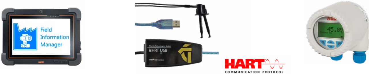
Figure 7: Field Information Manager with HART modem and field device
